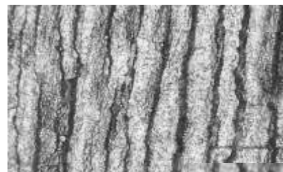
Fig.14 Surface morphology of the coating after thermal shock test
