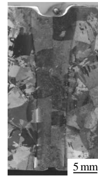
Fig.1 Appearance of ZTC4 plate weld by electron beam welding (20 mm thickness)
