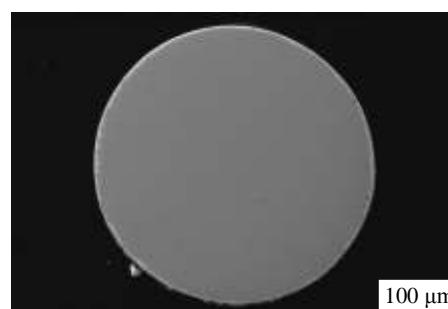
Fig.1 Cross-section photograph of \text{Zr}_{41.2}\text{Ti}_{13.8}\text{Cu}_{12.5}\text{Ni}_{10}\text{Be}_{22.5} BMG-coated Q195 steel wire
