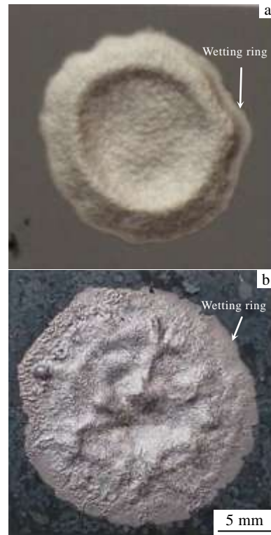
图 5 1050 °C/10 min 时钎料对 TiAl 板的宏观润湿照片 Fig.5 Macroscopical photos of wetting of the crystalline (a) and amorphous (b) fillers to TiAl at 1025 °C for 10 min
