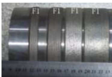
Fig.3 Morphology of shaft section by laser cladding
