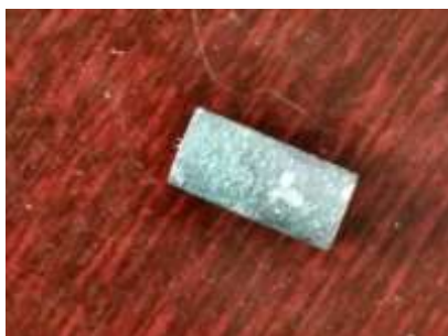
图 4 1#试样宏观腐蚀形貌图 Fig.4 Macro corrosion morphology of sample 1#
