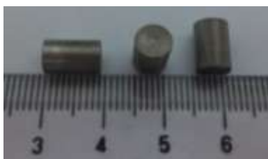
图 2 商业纯钛压缩试样 Fig.2 Sample for compression test
