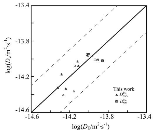
Fig.2 Comparison between the main calculated interdiffusion coefficients of the fcc Co-Cr-V system at 1473 K and the experimental values (dashed lines refer to the diffusion coefficients with a factor of 2 or 0.5 from the model-predicted ones)
