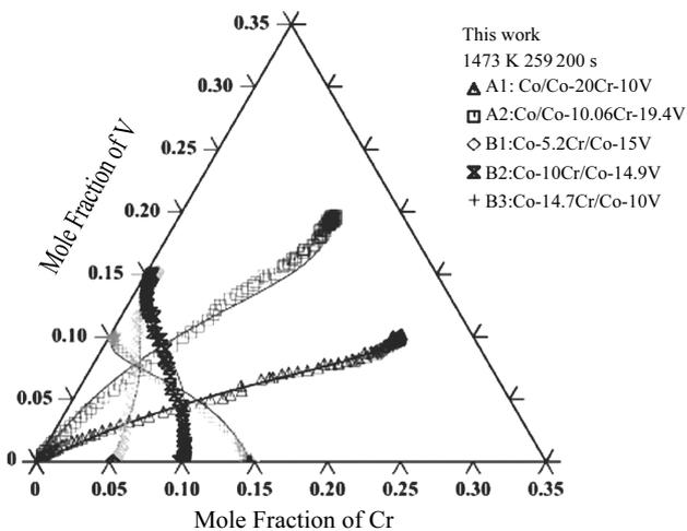
Fig.4 Calculated diffusion paths for various ternary Co-Cr-V diffusion couples annealed at 1473 K for 259200 s, compared with the experimental data measured in this work
