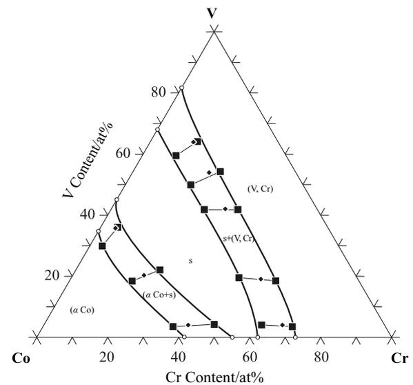
**Fig.1** Calculated isothermal section at 1473 K in the Co-Cr-V system using the thermodynamic parameters of Zhao et al<sup>[26]</sup>
