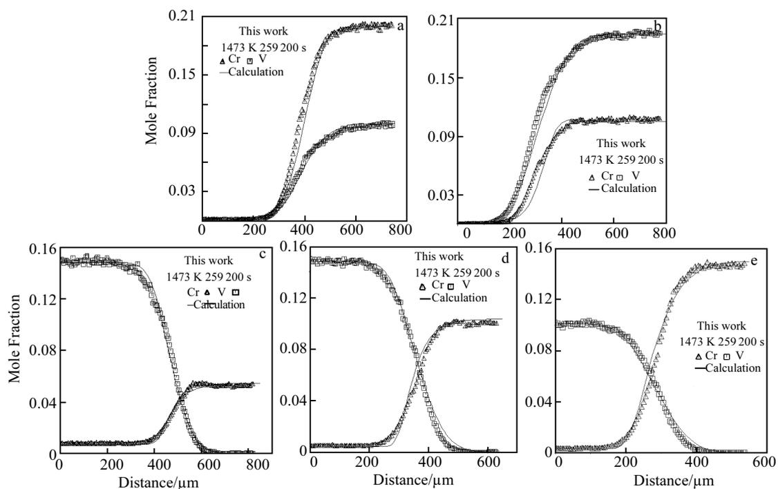
Fig.3 Comparison between the calculated and the measured concentration profiles of Co/Co-20Cr-10V (a), Co/Co-10.06Cr-19.4V (b), Co-5.2Cr/Co-15V (c), Co-10Cr/Co-14.9V (d), and Co-14.7Cr/Co-10V (e) diffusion couple annealed at 1473 K for 259 200 s
