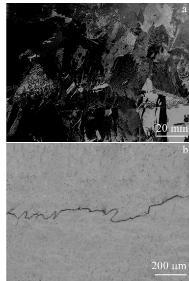
Fig.1 Microstructures of EB-Ti captured by stereo microscope (a) and metallurgical microscope (b)
