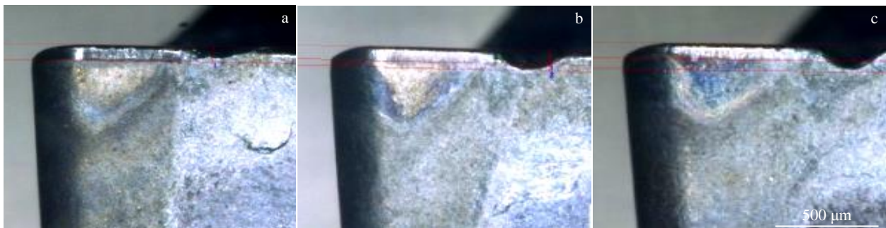
Fig.7 Morphologies of worn flank edges of the TNMG160404 inserts sintered at different temperatures during continuous cutting: (a) 1410 °C, (b) 1470 °C, and (c) 1490 °C
