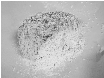
图 2 8YSZ 粉体喂料的宏观形貌 Fig.2 Macro morphology of 8YSZ powder feed
