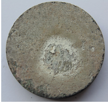
Fig.10 Macrograph of the ZrB_2 - ZrC - SiC coated C/C composites after ablation under the plasma flame for 60 s
