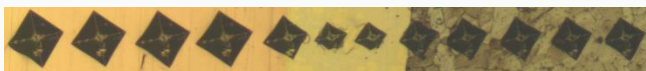
图 7 70% CuSn 合金粉复合药芯银钎料钎焊的接头显微硬度压痕 Fig.7 Micro-hardness indentation morphology of joint brazed with composite flux-cored silver brazing filler metal with 70% CuSn alloy powder
