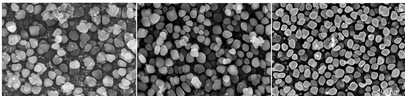
Fig.2 Morphologies of  $\gamma'$  particles after long-term aging at 680 °C (a), 700 °C (b), and 730 °C (c) for 3000 h
