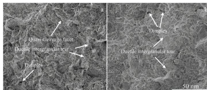
Fig.6 Tensile fractographs at 650 °C of U720Li superalloys aged at 730 °C for 500 h (a) and 3000 h (b)
