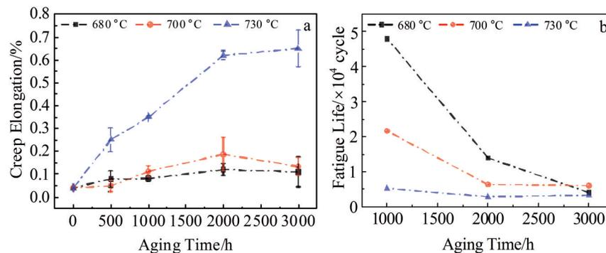
Fig.7 Elongation after creep at 625 °C/730 MPa (a) and fatigue life at 650 °C/1250 MPa with strain amplitude of 0.05 and loading frequency of 0.33 Hz (b) for U720Li superalloys after long-term aging
