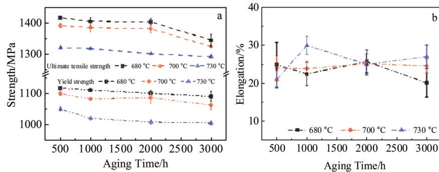
Fig.5 Tensile properties at 650 °C of U720Li superalloy under different aging conditions: (a) yield strength and ultimate tensile strength; (b) elongation
