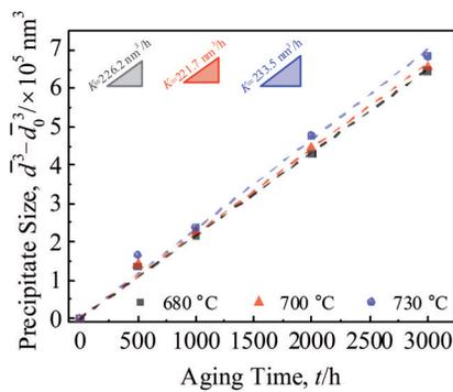
Fig.3 Relationship of precipitate size ( $\bar{d}^3 - \bar{d}_0^3$ ) and aging time ( $t$ ) during long-term aging at 680, 700, and 730 °C
