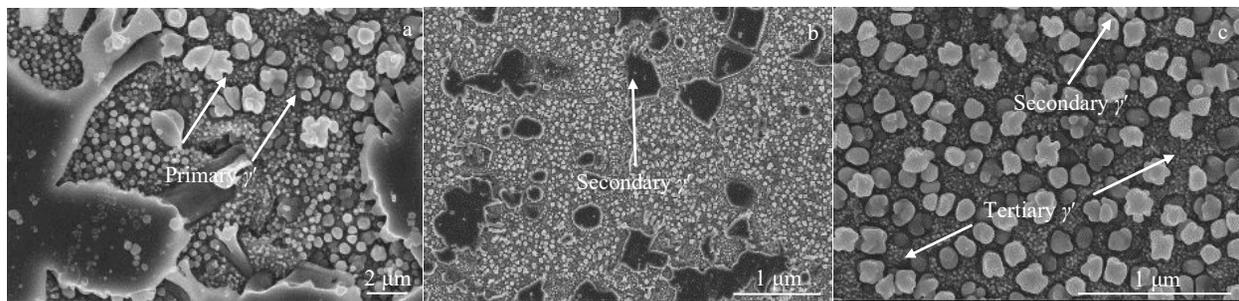
Fig.1 Morphologies of primary  $\gamma'$  phase (a), secondary  $\gamma'$  phase (b), and tertiary  $\gamma'$  particles (c) in U720Li superalloy before long-term aging
