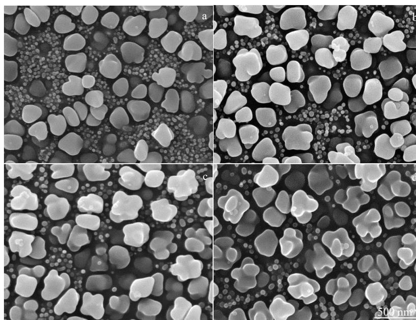
Fig.4 Morphologies of  $\gamma'$  particles after aging at 730 °C for 500 h (a), 1000 h (b), 2000 h (c), and 3000 h (d)
