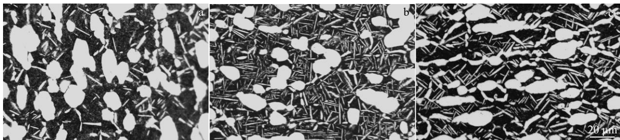
Fig.5 Final microstructures of TA15 alloys after processes of T_1/0.1 s -1 /60%/WQ+930 °C/1 h/AC+550 °C/5 h/AC at different deformation temperatures: (a) T_1=965 °C, (b) T_1=970 °C, and (c) T_1=975 °C
