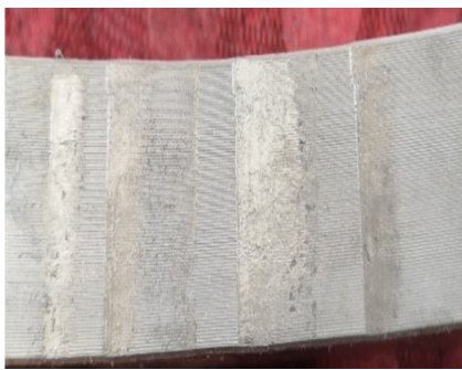
Fig.13 “Steps” caused by the cold bulging process
