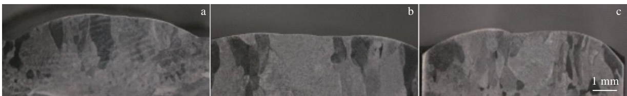
图 8 不同焊道间距搭接效果 Fig.8 Lap effect of different weld spacing: (a) 4.8 mm, (b) 5.3 mm, and (c) 5.8 mm
