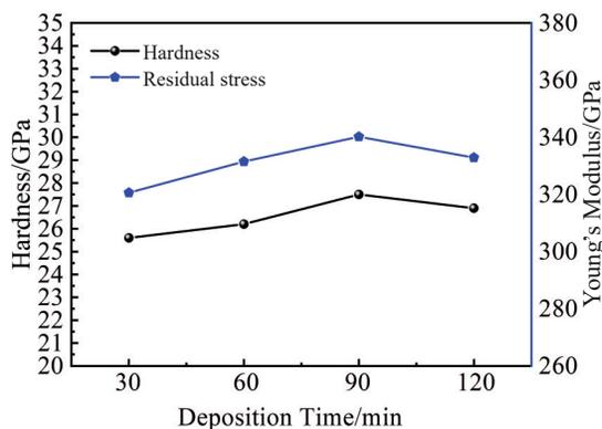
Fig.5 Hardness and Young's modulus of TiN coatings under different deposition time conditions
