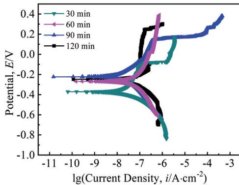
Fig.8 Electrochemical polarization curves of TiN coatings under different deposition time conditions
