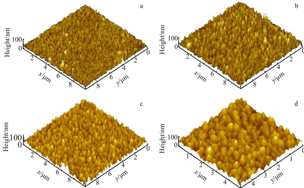
Fig.2 AFM three-dimensional morphologies of TiN coatings under different deposition time conditions: (a) 30 min, (b) 60 min, (c) 90 min, and (d) 120 min
