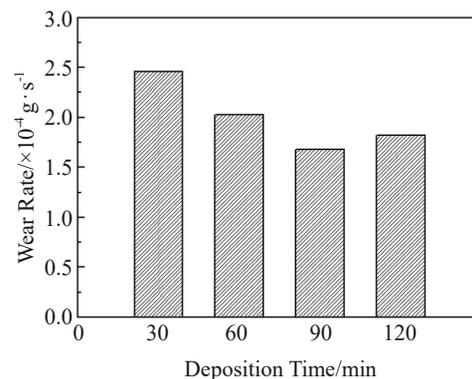
Fig.7 Wear rates of TiN coatings under different deposition time conditions
