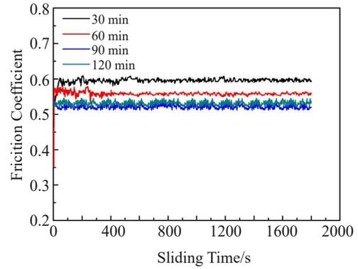
Fig.6 Friction coefficient curves of TiN coatings under different deposition time conditions
