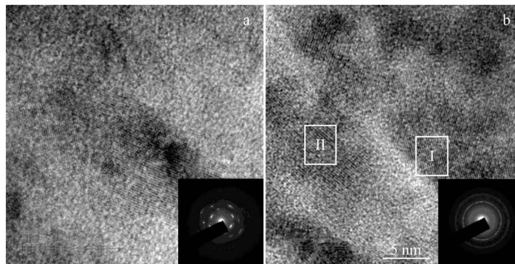
Fig.3 High-resolution TEM images with corresponding SAED patterns of TiN coatings after deposition for 30 min (a) and 120 min (b)
