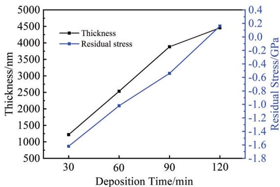
Fig.4 Thickness and residual stress of TiN coatings under different deposition time conditions
