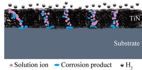
Fig.9 Schematic diagram of corrosion mechanism of TiN coating
