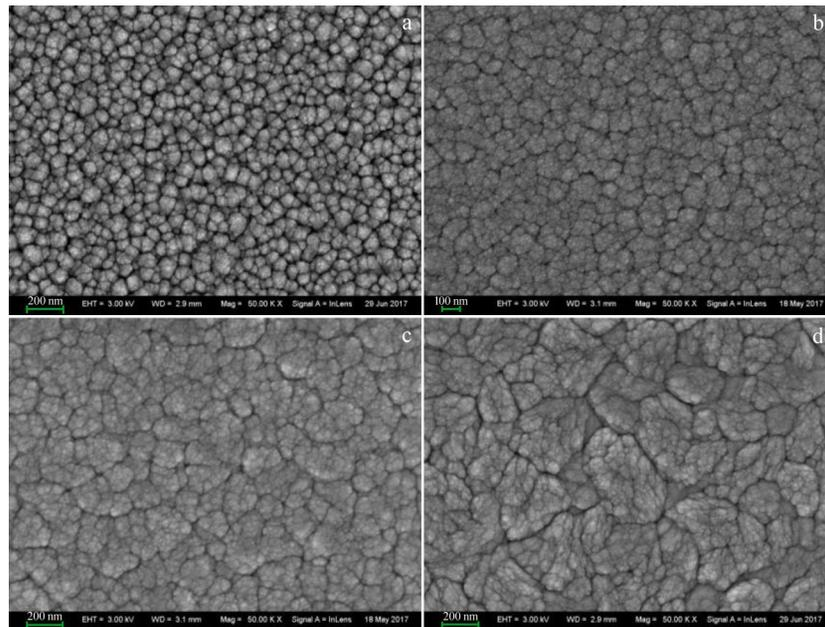
Fig.1 SEM surface microstructures of TiN coatings under different deposition time conditions: (a) 30 min, (b) 60 min, (c) 90 min, and (d) 120 min
