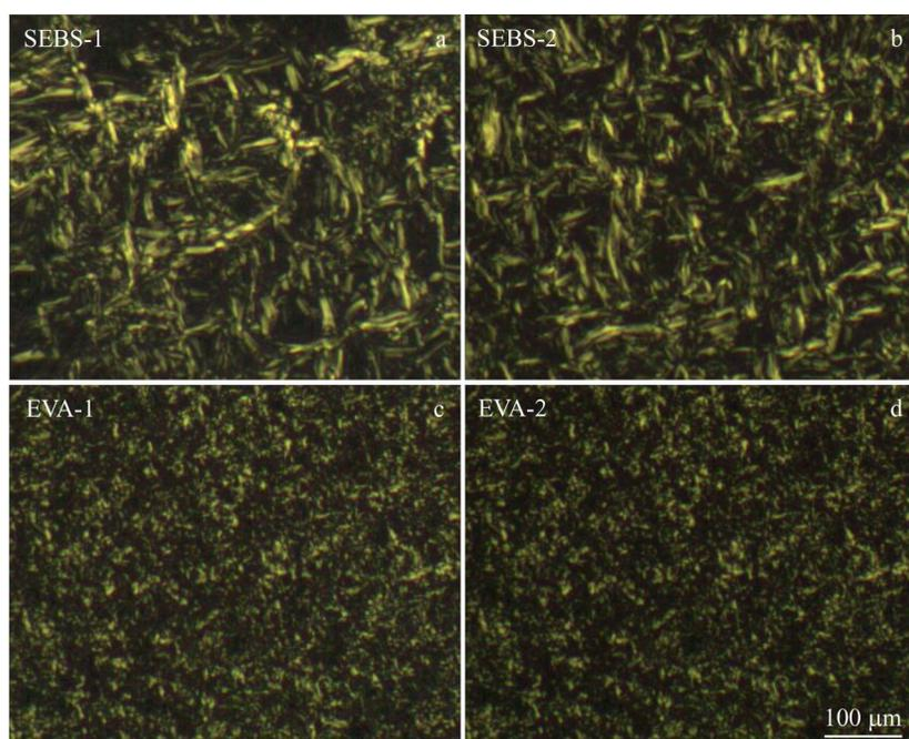
Fig.3 OM images of microstructure of resin-modified paraffin waxes: (a) SEBS-1, (b) SEBS-2, (c) EVA-1, and (d) EVA-2
