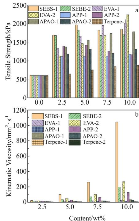
Fig.5 Effect of modifier content on tensile strength (a) and kinematic viscosity (b) of modified paraffin waxes
