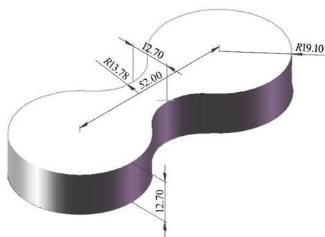
Fig.1 Paraffin wax specimen used for tensile strength test
