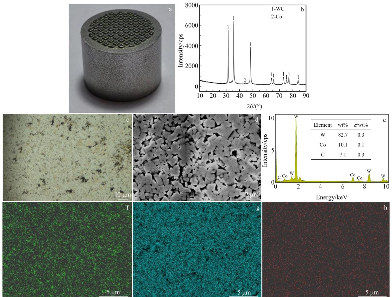
Fig. 9 Appearance (a), XRD pattern (b), OM image (c), SEM image (d), EDS analysis result (e) and EDS mappings of element Co (f), W (g) and C (h) of surface of deep well-shaped WC-Co alloy block made in industry
