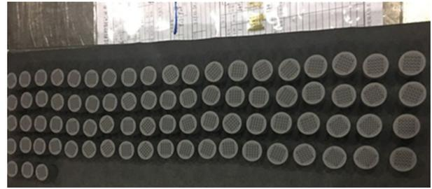
Fig. 8 Green compacts produced by the forming agent of modified paraffin waxes
