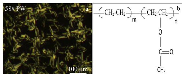
Fig.2 OM image of morphology of 58# paraffin wax (a) and structure of EVA resin (b)
