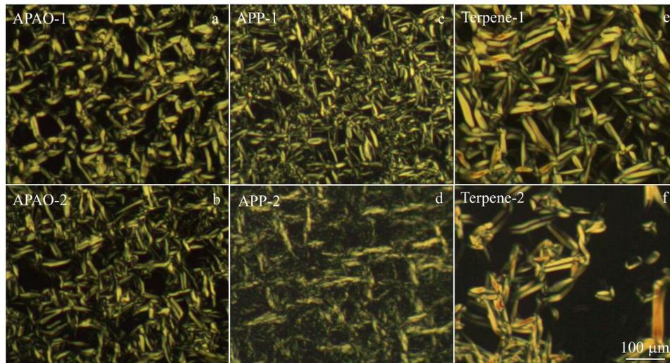
Fig.4 OM images of microstructure of resin-modified paraffin waxes: (a) APAO-1, (b) APAO-2, (c) APP-1, (d) APP-2, (e) Terpene-1, and (f) Terpene-2
