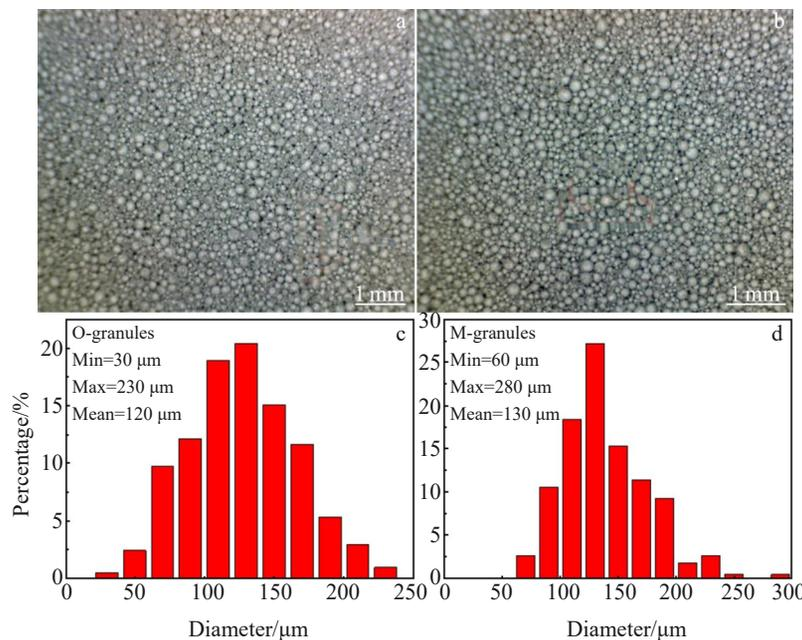
Fig. 7 Appearances (a–b) and size distributions (c–d) of sprayed granules made from O-granules (a, c) and M-granules (b, d)
