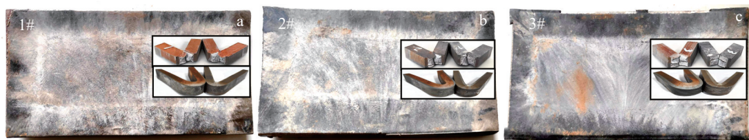
Fig.5 Composite plates with different flyer plate thicknesses after explosion and mechanical tests: (a) 1 mm; (b) 2 mm; (c) 4 mm
