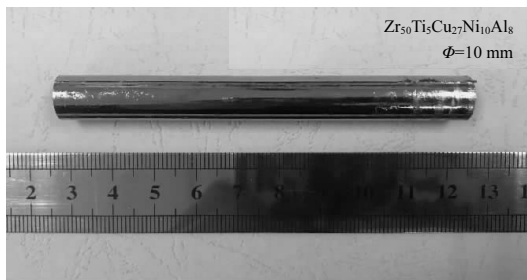
Fig.2 Macroscopic feature of the Zr50 metallic glass with the diameter of 10 mm
