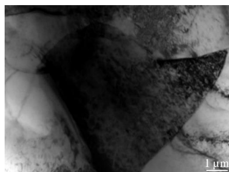
Fig.9 TEM image of \alpha -Mg phase in ECAPed 8 pass Mg-9Li alloy [169]
