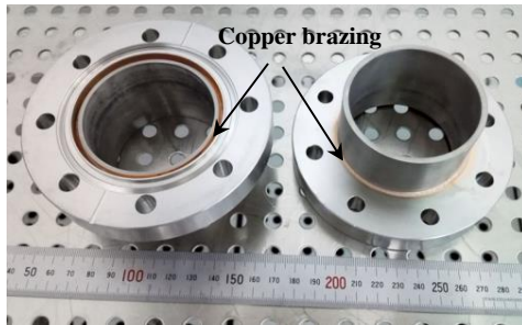
Fig.6 Transition joints after brazing
