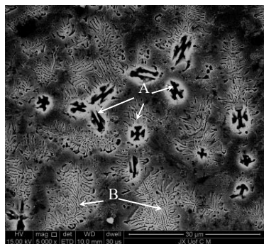
Fig.3 Microstructure of 15wt%Mg 2 Si/Al with laser power of 900 W
