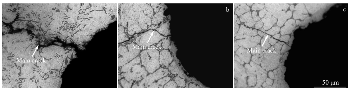
Fig.10 Microstructures near the gap region of specimen A (a), specimen B (b), and specimen C (c) after thermal fatigue cycles of N=24\ 500
