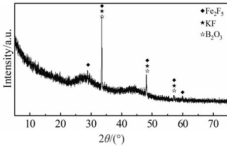
Fig.8 XRD pattern of reaction product of oxide film and mixed flux of  $H_3BO_3$  and  $KF$  at 700 °C
