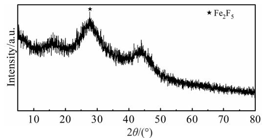
Fig.10 XRD pattern of reaction product of oxide film and FB3-F flux at 700 °C
