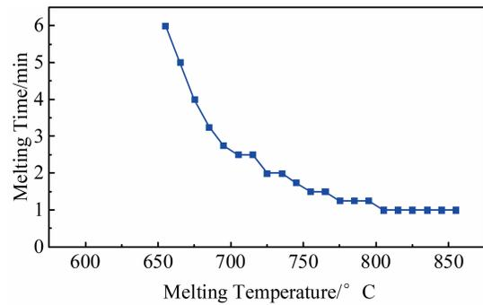
Fig.2 Relationship between melting time and melting temperature
