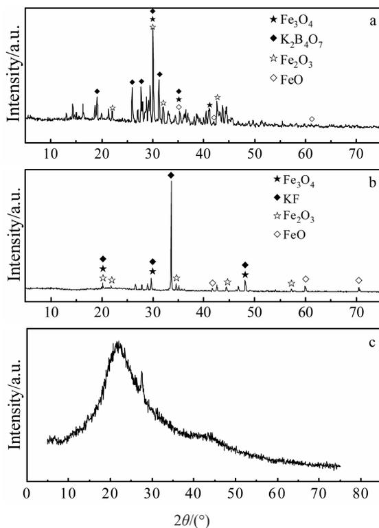
Fig.5 XRD patterns of reaction products of oxide film and different flux at 700 °C: (a) K<sub>2</sub>B<sub>4</sub>O<sub>7</sub>, (b) KF, and (c) H<sub>3</sub>BO<sub>3</sub>
