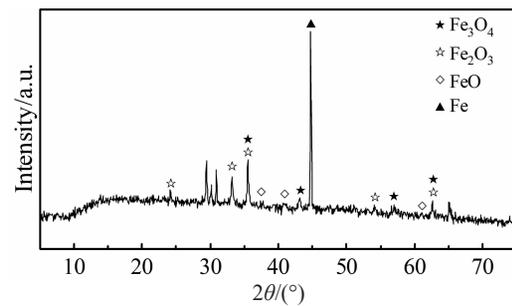
Fig.3 XRD pattern of oxide film on Q235 steel plate at 700 °C
