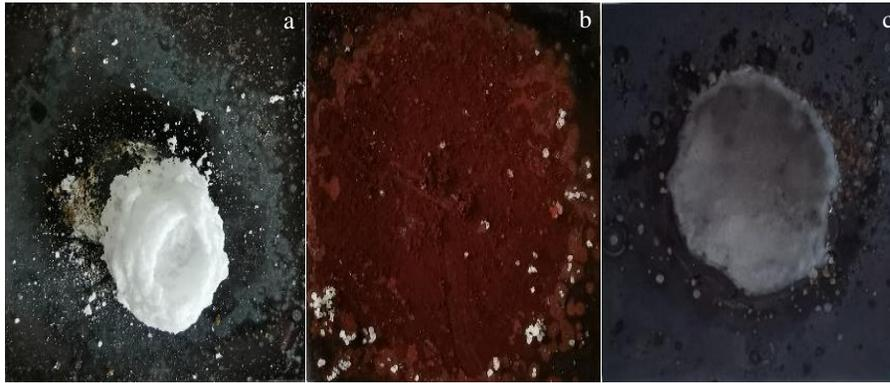
Fig.4 Surface morphologies of Q235 steel plate after reaction with different flux at 700 °C: (a) K<sub>2</sub>B<sub>4</sub>O<sub>7</sub>, (b) KF, and (c) H<sub>3</sub>BO<sub>3</sub> at 1:1 scale
