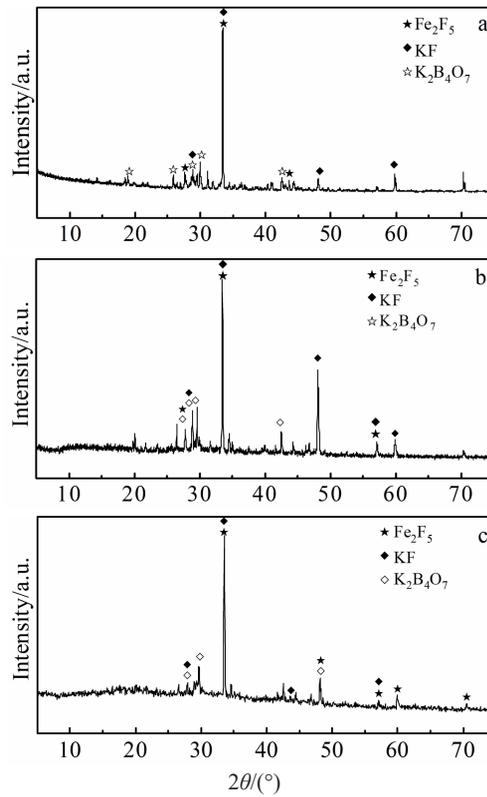
Fig.9 XRD patterns of reaction product of oxide film and mixture flux of  $K_2B_4O_7$  and  $KF$  with different mass ratios: (a) 10: 3, (b) 7:3, and (c) 6:4
