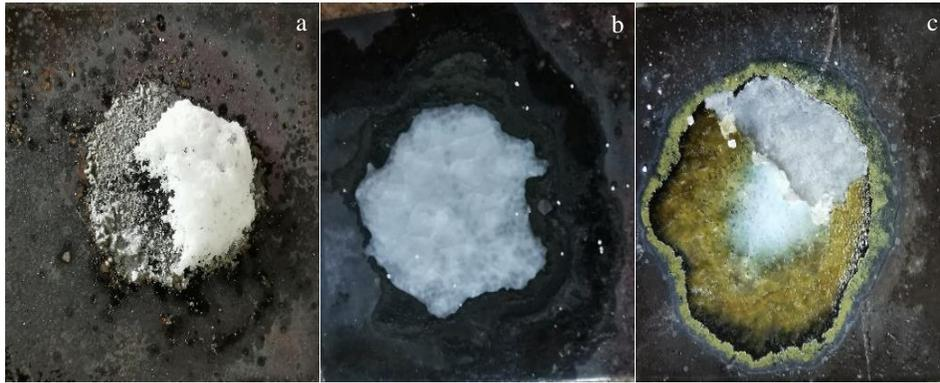
Fig.6 Surface morphologies of Q235 steel plate after reaction with different mixed flux at 700 °C: (a)  $K_2B_4O_7+H_3BO_3$ , (b)  $KF+H_3BO_3$ , and (c)  $KF+K_2B_4O_7$  at 1:1 scale
