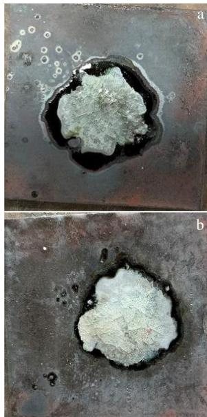
Fig.1 Surface morphologies of Q235 steel plate after film removal at 800 °C (a) and 700 °C (b) at 1:1 scale
