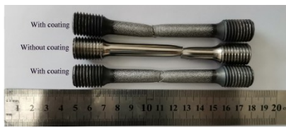
Fig.11 Fracture appearances of Ti6Al4V alloy specimens with and without oxygen-carbon co-cemented coating
