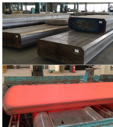
图 1 EB 炉熔炼扁锭与直轧板材
