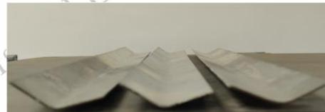
Fig. 8 Magnesium alloy roll-formed parts
