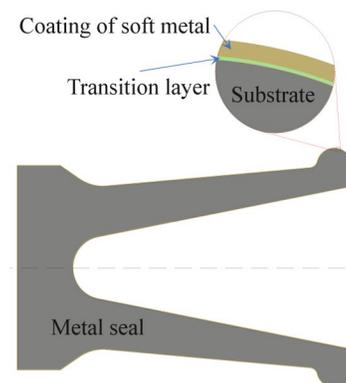
Fig.1 Sketch of coating of soft metal for metal seal
