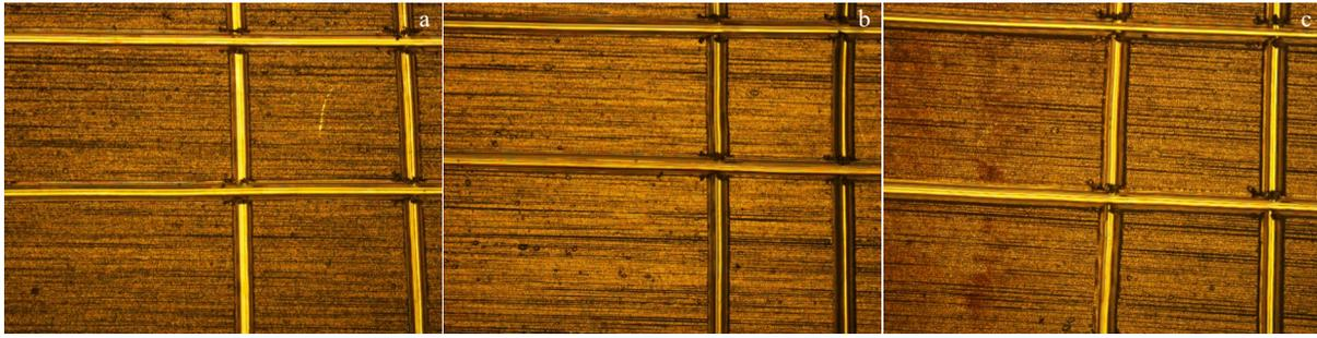
Fig.11 Results of cross-cut test for GH4169-Cu with different thicknesses of Ag coating: (a) 20  $\mu\text{m}$ , (b) 30  $\mu\text{m}$ , and (c) 40  $\mu\text{m}$
