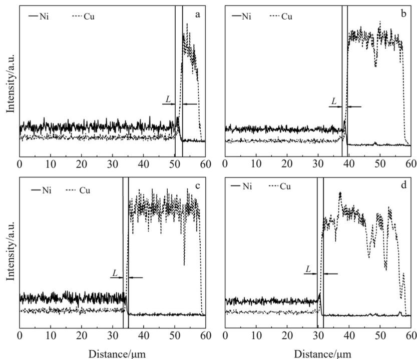
Fig.5 EDS line scan results for GH4169 with different thicknesses of Cu coating: (a) 10  $\mu\text{m}$ , (b) 20  $\mu\text{m}$ , (c) 30  $\mu\text{m}$ , and (d) 40  $\mu\text{m}$
