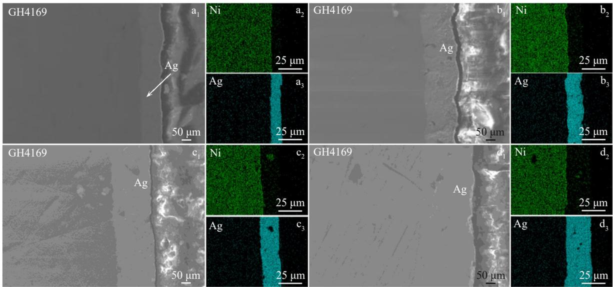
Fig.3 SEM interface morphologies ( $a_1-d_1$ ) and EDS element mappings ( $a_2-d_2$ ,  $a_3-d_3$ ) of GH4169 with different thicknesses of Ag coating: ( $a_1-a_3$ ) 10  $\mu\text{m}$ , ( $b_1-b_3$ ) 20  $\mu\text{m}$ , ( $c_1-c_3$ ) 30  $\mu\text{m}$ , and ( $d_1-d_3$ ) 40  $\mu\text{m}$
