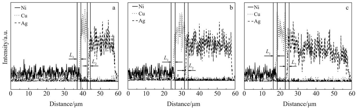
Fig.7 EDS line scan results for GH4169-Cu with different thicknesses of Ag coating: (a) 20  $\mu\text{m}$ , (b) 30  $\mu\text{m}$ , and (c) 40  $\mu\text{m}$
