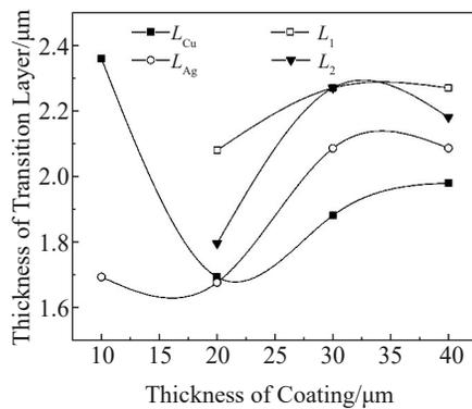
Fig.8 Influence of thickness of coatings on transition layer
