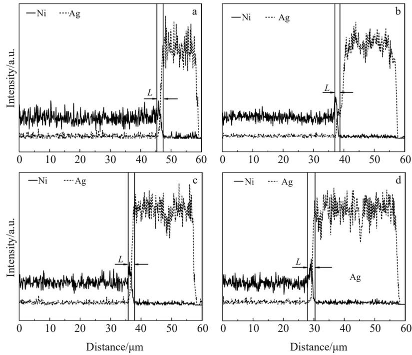
Fig.6 EDS line scan results for GH4169 with different thicknesses of Ag coating: (a) 10  $\mu\text{m}$ , (b) 20  $\mu\text{m}$ , (c) 30  $\mu\text{m}$ , and (d) 40  $\mu\text{m}$
