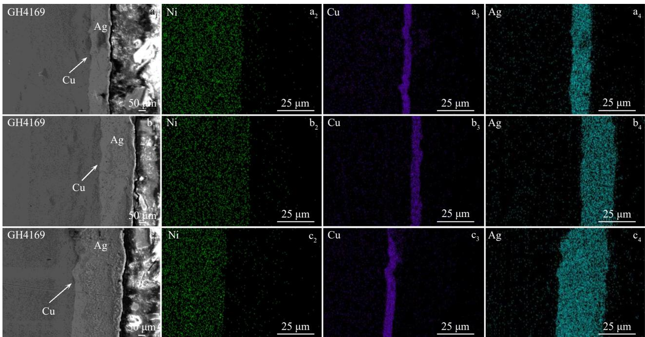
Fig.4 SEM interface morphologies ( $a_1-c_1$ ) and EDS element mappings ( $a_2-c_2$ ,  $a_3-c_3$ ,  $a_4-c_4$ ) of GH4169-Cu with different thicknesses of Ag coating: ( $a_1-a_4$ ) 20  $\mu\text{m}$ , ( $b_1-b_4$ ) 30  $\mu\text{m}$ , and ( $c_1-c_4$ ) 40  $\mu\text{m}$
