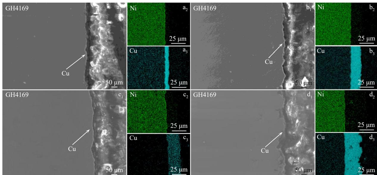
Fig.2 SEM interface morphologies (a<sub>1</sub>–d<sub>1</sub>) and EDS element mappings (a<sub>2</sub>–d<sub>2</sub>, a<sub>3</sub>–d<sub>3</sub>) of GH4169 with different thicknesses of Cu coating: (a<sub>1</sub>–a<sub>3</sub>) 10  $\mu\text{m}$ , (b<sub>1</sub>–b<sub>3</sub>) 20  $\mu\text{m}$ , (c<sub>1</sub>–c<sub>3</sub>) 30  $\mu\text{m}$ , and (d<sub>1</sub>–d<sub>3</sub>) 40  $\mu\text{m}$
