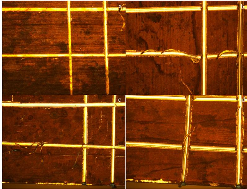
Fig.9 Results of cross-cut test for GH4169 with different thicknesses of Cu coating: (a) 10  $\mu\text{m}$ , (b) 20  $\mu\text{m}$ , (c) 30  $\mu\text{m}$ , and (d) 40  $\mu\text{m}$
