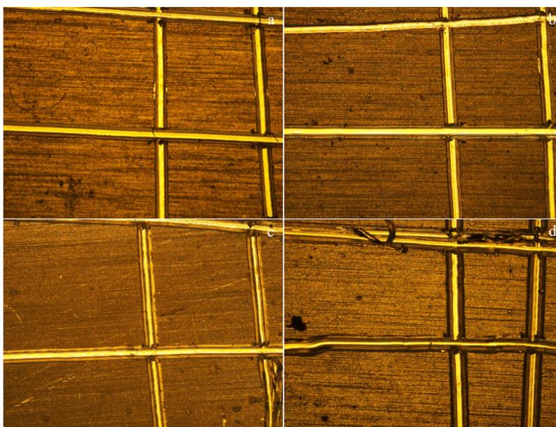
Fig.10 Results of cross-cut test for GH4169 with different thicknesses of Ag coating: (a) 10  $\mu\text{m}$ , (b) 20  $\mu\text{m}$ , (c) 30  $\mu\text{m}$ , and (d) 40  $\mu\text{m}$
