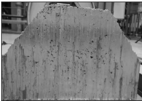
图9 采用优化凸模压制的 TC4 钛合金电极块 Fig. 9 TC4 titanium alloy electrode block pressed by optimized punch
