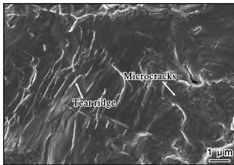
图7 TC4钛合金试样疲劳断口瞬断区撕裂棱与微裂纹的形貌 Fig.7 Morphologies of tear corrugations and microcracks in transient fracture zone of TC4 titanium alloy specimen
