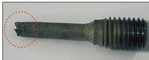
图2 高温持久异常断裂试样照片 Fig.2 Photo of high temperature endurance abnormal fracture specimen
