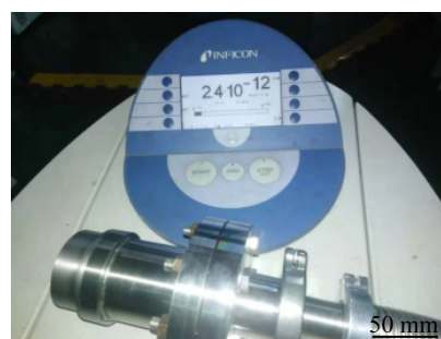
Fig.11 Leak check for the joint
