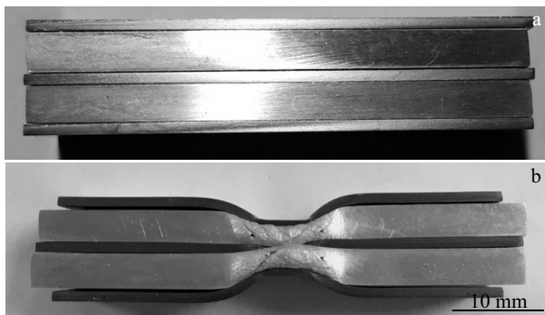
Fig.3 Compression specimen of TA1/AZ31B multi-layer composites: (a) before compressing and (b) after compressing
