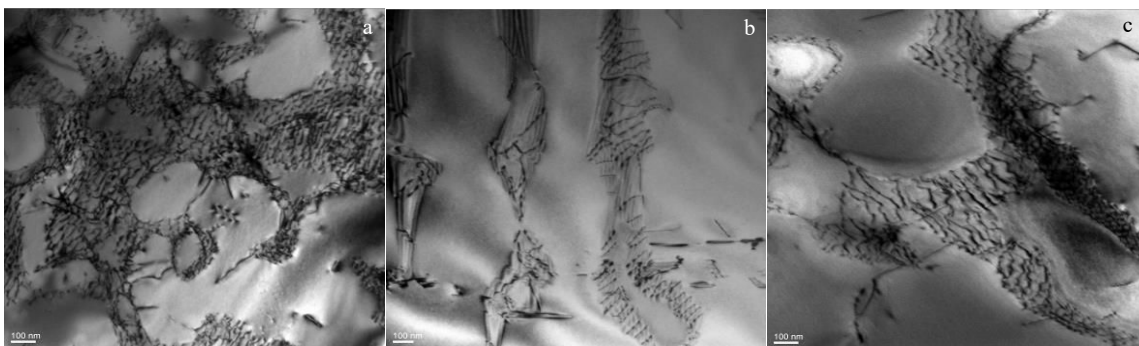
Fig.5 Creep fracture microstructures of DD15 alloy with different orientations at 980 °C/300 MPa: (a) [001], (b) [011], and (c) [111]
