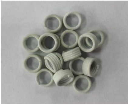
Fig.2 Environmentally friendly ring-shaped flux-coated brazing materials [35]
