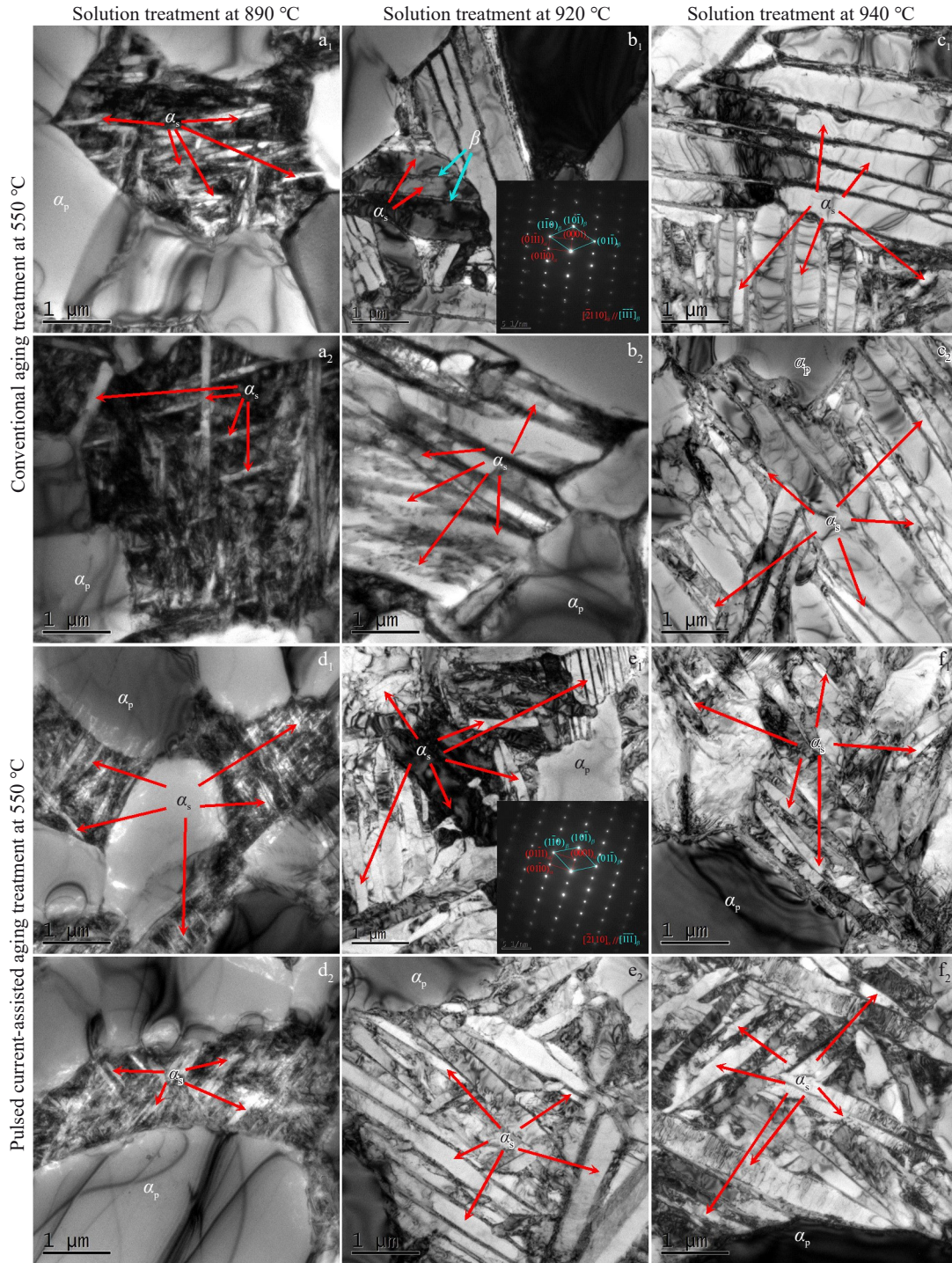
Fig.7 TEM images of different samples: (a 1 , a 2 ) S890A550, (b 1 , b 2 ) S920A550, (c 1 , c 2 ) S940A550, (d 1 , d 2 ) S890EA550, (e 1 , e 2 ) S920EA550, and (f 1 , f 2 ) S940EA550
