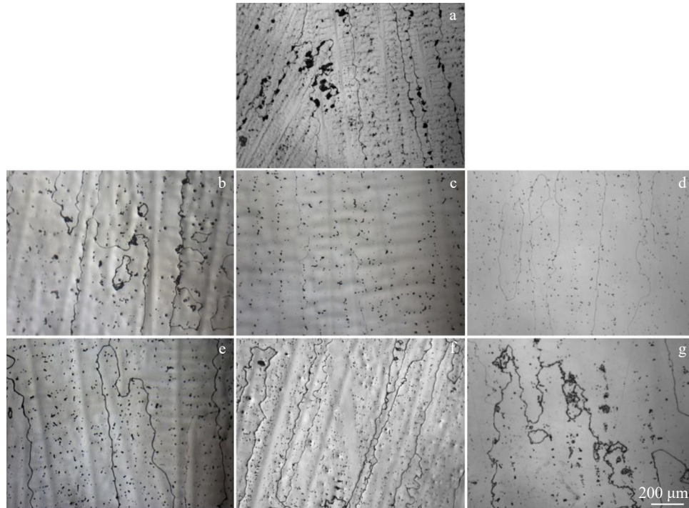
Fig.4 OM morphologies of GH3535-0.08Y alloys with metallographic etching before (a) and after homogenization at 1150 °C (b–d) and 1188 °C (e–g) for 2 h (b, e), 5 h (c, f), and 10 h (d, g)
