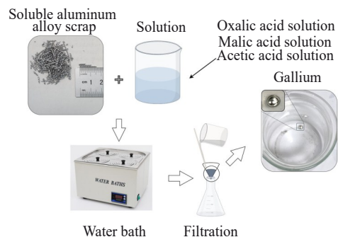
图 1 从 Al-Ga-Mg-Sn 中回收 Ga 的工艺流程图 Fig.1 Process flowchart for Ga recovery from Al-Ga-Mg-Sn
