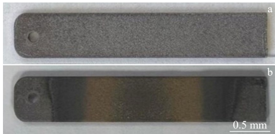
Fig.13 Macroscopic morphologies of Si-Cr-Ti-Zr coatings on Ta12W alloy with MAO pretreatment at 400 V before (a) and after (b) oxidation at 1600 °C for 5 h
