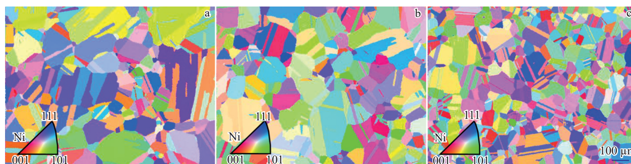
Fig.6 IPF maps showing the grain morphology of solution-treated GH4750 alloy with different C contents: (a) 0.024wt%, (b) 0.042wt%, and (c) 0.082wt%
