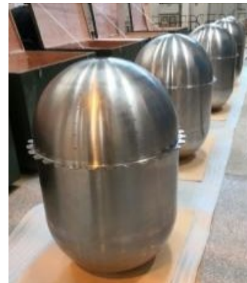
Fig.16 Appearance of surface tension tank for propellant storage
