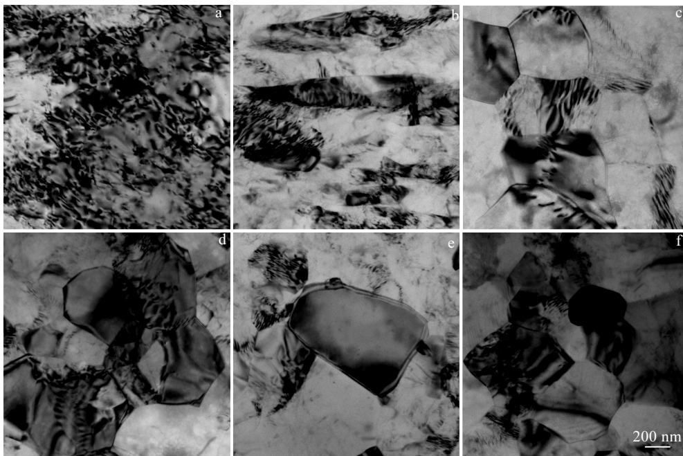
Fig.2 TEM micrographs in the different regions of the samples processed by HPT for various revolutions: (a) region I, (b) region II, and (c) region III for 1 revolution; region III for 3 (d), 5 (e) and 20 (f) revolutions
