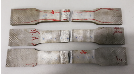
图 7 Al-5.6Zn-3.5Ni-2Mg-1Cu 铝合金焊接接头的断口形貌 Fig.7 Tensile fracture morphology of Al-5.6Zn-3.5Ni-2Mg-1Cu aluminum alloy welded joint
