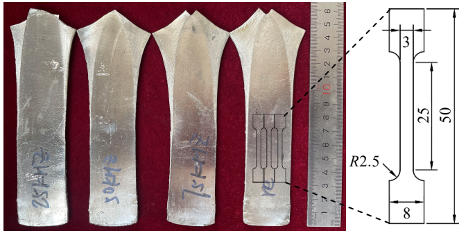
图2 AZ31B 镁合金复合板试样外观及拉伸试样尺寸和取样位置 Fig.2 Appearance of AZ31B magnesium alloy composite plates and the size and position of tensile sample
