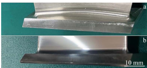
Fig.10 Appearances of blade root before (a) and after (b) polishing
