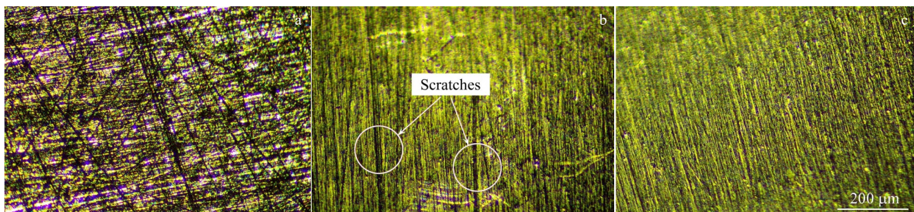
Fig.7 Comparison of surface morphologies before polishing (a) and polished with inelastic magnetic tool (b) and elastic magnetic tool (c)
