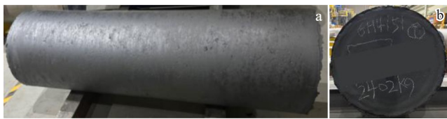
图2 三联熔炼 \Phi 508 mm 规格 GH4151 合金铸锭 Fig.2 Triple-melted \Phi 508 mm ingot of GH4151 superalloy: (a) peripheral and (b) top surfaces
