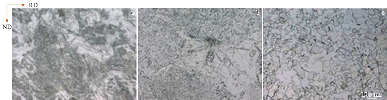
Fig. 4 Microstructures of TA1/304 composite plates at different states: (a) Origin; (b) 550 °C; (c) 650 °C
