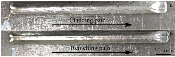
Fig.3 Coating appearances and characteristics of specimens W1 (a) and W4 (b)
